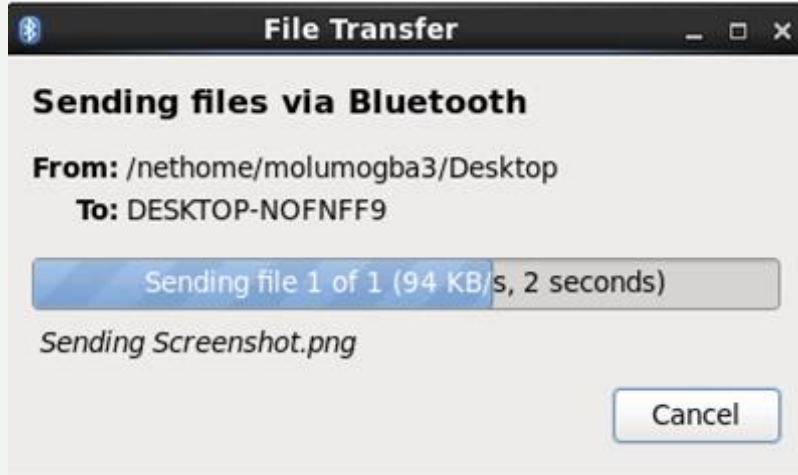
Figure 17. GUI indicating successful transfer of file after manually writing a new link key into linkkeys
